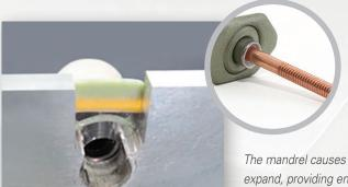
The mandrel causes the sleeve to expand, providing enough force to provide a secondary retention of the nutplate in the structure.
